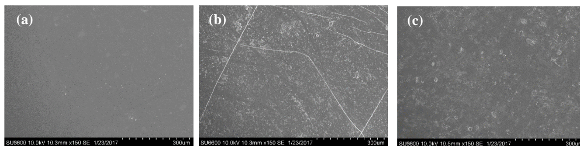
Figure 3.20 SEM micrograph of 75% (w/w) Poly(St-co-N-Cin) copolymer film (a) before outdoor weathering ( \times 150 ) (b) after 80 days of outdoor weathering ( \times 150 ) (c) Polystyrene film after 80 days of outdoor weathering ( \times 150 ).
