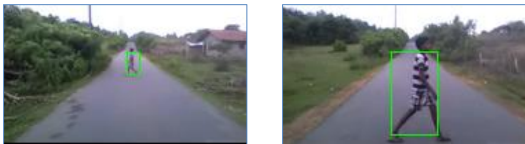
Figure 5: Two safe scenarios for pedestrian crossing the road; a distant pedestrian and a near pedestrian.
