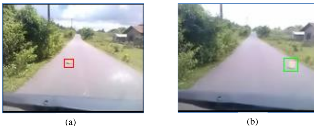
Figure 3: (a) The object is tracked using a red boundary box since it has a potential for a collision. (b) The object which does not cause a collision is tracked using a green boundary box
