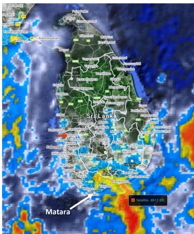
Figure 8. Cloud distribution on the 1st May 2013 at 16:00 UTC. The areas in red denote cooler regions which are considered to be as the origins of lightning activity. According to the scale the approximate distance between the charge centre and measurement site was 80 km. (image obtained from http://www.wunderground.com )
