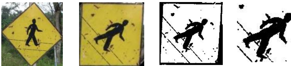
Figure 5: (a) Identified road sign region (b) Extracted region after Radon transformation (c) Binarized image (d) Cropped image (96x96)
