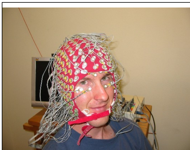
Figure 2.37: EEG recording using an electrode-cap
